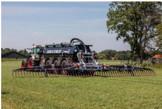
Image 3: BlackBird Pro trailing shoe linkage, here in a working width of 15 meters.
