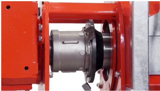
Image 5: Close-up: Settings can be flexibly adjusted during operation via the VarioAdjust system depending on the desired dry matter content.
