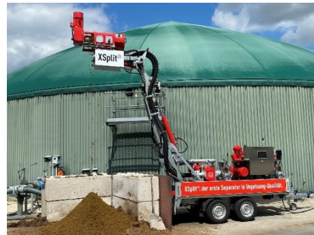
Image 4: The XSplit press screw separator – innovative separation technology, available as a system solution (shown) or as a stand-alone version.
